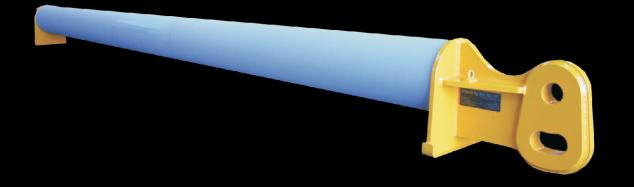
The Maxilug 145 allows users to create their own custom length, medium-lift spreader bar utilizing these heavy duty end units. Designed to accomodate readily available line pipe, Maxirig can supply the units as is or with various pipe lengths to facilitate lift spans from 2 metres up to 13 metres.
