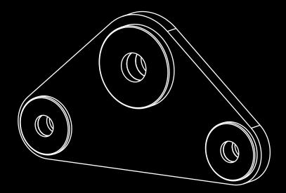
When using multiple sling legs this device provides a means of equalising forces within the legs. Connection is made via standard Grade "S" bow shackle and can be used with chain, wire rope or synthetic slings. Ideal in compensating for diferences in load lift points and sling lengths.
