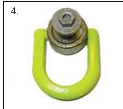
4. Put the screw into the bush.
