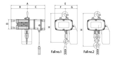
A 715mm B 340mm C 375mm D 220mm E 570mm F 270mm G 260mm H 1100mm
