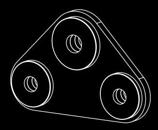
When using multiple sling legs this device provides a means of equalising forces within the legs. Connection is made via standard Grade "S" bow shackle and can be used with chain, wire rope or synthetic slings. Ideal in compensating for diferences in load lift points and sling lengths.
