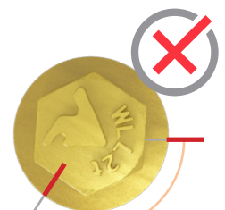
D - Greater than 90° Report to authority on site.
