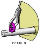
DETAIL B SCALE 1 : 5 Cabinet sub frames typically have 50mm holes incorporated and the lifting bars are 42mm.
